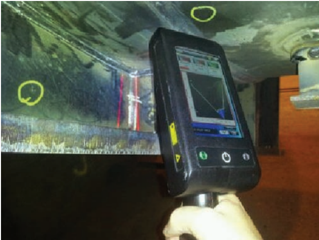
Fig. 3 — Checking weld size on heavy-plate pressure vessels.
